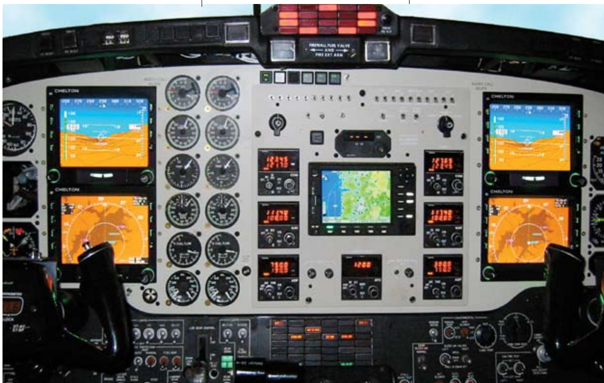
Four-screen install on a King Air 300
