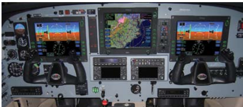
From the pilot's perspective, the Avidyne Entegra, such as the one in this Piper panel, functions as a true IFD.
