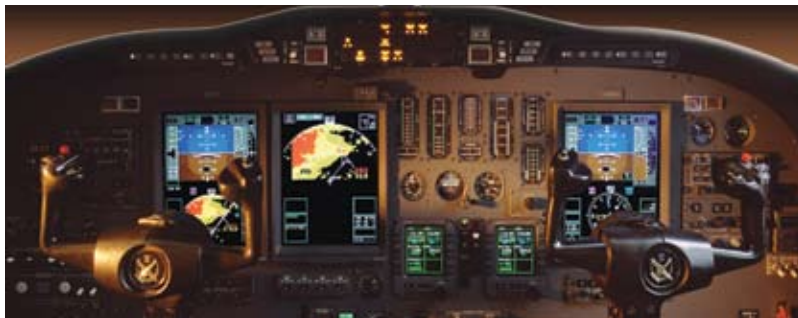
The Honeywell Primus Epic is a truly integrated IFD with all sensors, radios and others items in a central unit.
