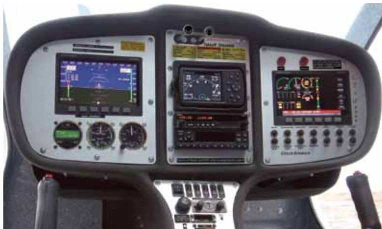
A good percentage of new light-sport aircraft, such as this Flight Design CTLS, sport the same avionics package: Dynon glass, Garmin avionics, and a handheld GPS 396/496 with XM weather in an AirGizmo panel-mount.
