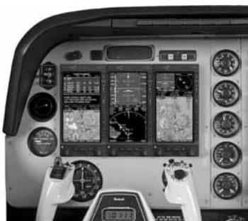
The Aspen Avionics Evolution flight displays installed in a Beechcraft Bonanza. One, two or three individual EFD1000s replace the six-pack flight instruments.
