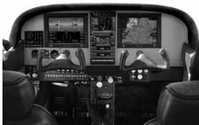
The Avidyne Entegra EXP5000 PFD and EX5000 MFD as a retrofit installation in a Cessna T210.
