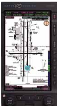
Aspen Avionics' Evolution with geo-referenced airport diagrams
